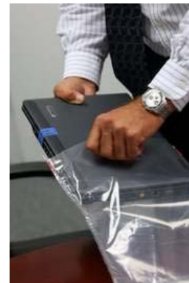
Robert Frucci, business development manager for CGM Applied Security Technologies Inc., places a laptop computer into a tamper-evident bag. If the bag is opened after it is sealed, it becomes discolored, alerting the owner to the tampering. (STAFF PHOTOS: BRADLEY J. PENNER) Buy this photo
